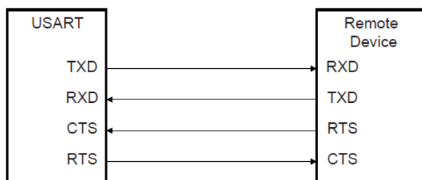
Figure 30-21: Hardware Handshake with Remote Devices
