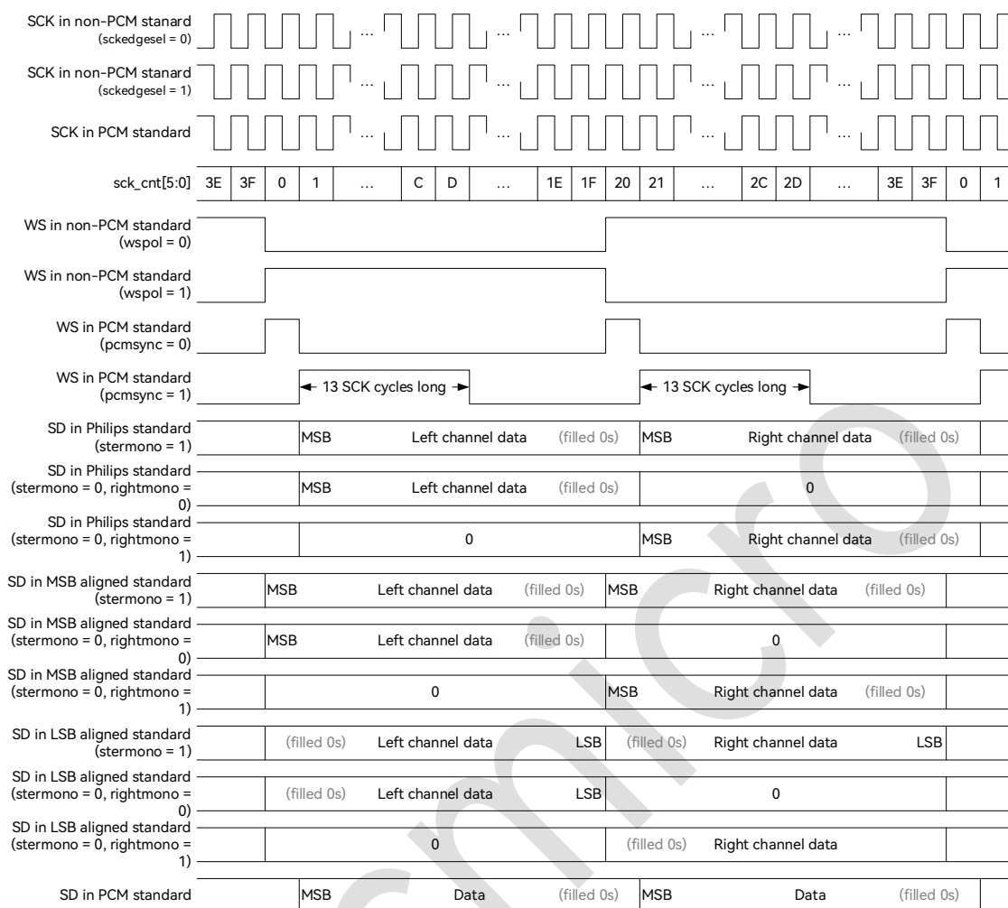
Figure 27-2: I2S Signal Waveform for 32-bit Channel
